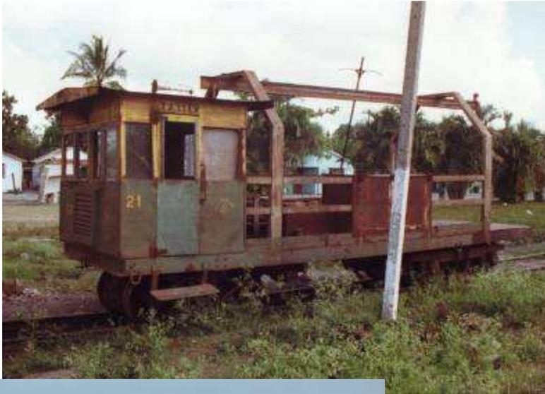
Figure 21 is a powered track maintenance car on Hermanos Ameijeiras mill, 3 ft gauge. This is a straight freight car conversion and looked to be out of use though it is sometimes difficult to tell. It is amazing what can be achieved with a battery and a can of fuel.
