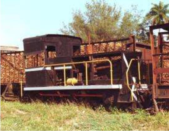
dating back to the 1870's. Fortunately the historic significance of this engine has now been recognized and it has had the diesel engine removed and its very moth eaten boiler put back in place. So far the cylinders have not been located! It is shown in Figure 9 in diesel mode out of use at Gregorio Arlee Manalich mill in 1999.
