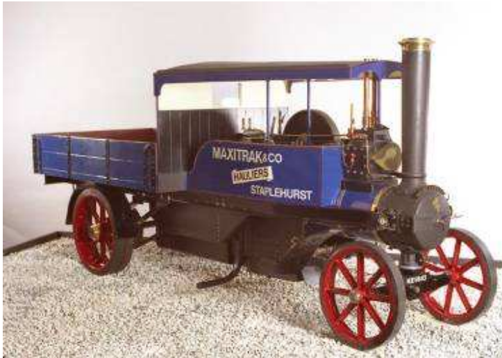
AVELING LORRY 3" scale, steam. Designed by A. Probyn Introduced 1993 Special order from 2003 onwards. A lorry based on the Aveling traction engine components, chain drive.
