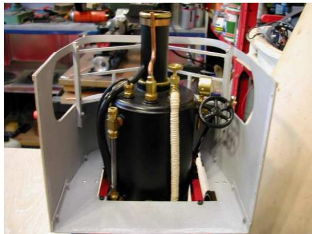
chassis members to take some 3mm cap head bolts to hold it down. The cab back, roof and bench seat were easily made up from the provided parts and fitted, only some sanding down to get a good fit. I had to remember that the roof is made to be simply lifted off for access to the boiler and therefore a loose fit is required to allow for paint etc.
