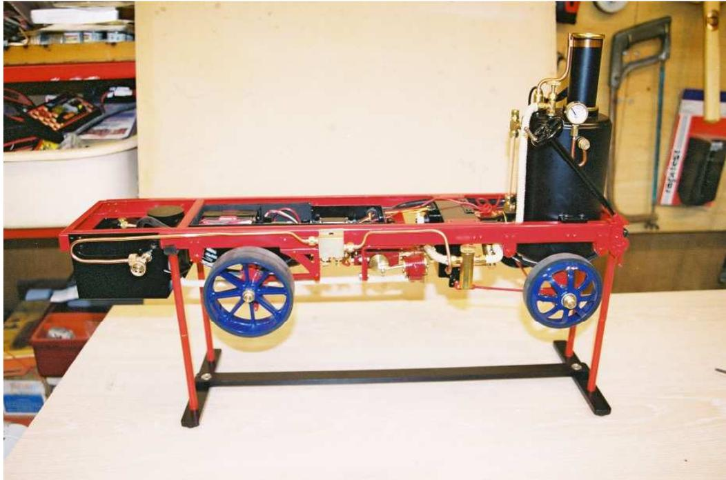
Extreme care must be used when using superglue here as apart from sticking ones fingers together, any glue spilt on the painted surface will destroy the finish and a repaint job will be necessary. Glue spilt on the rubber tyre isn't so bad as it can be rubbed down carefully with wet or dry paper once it has set and won't notice.
