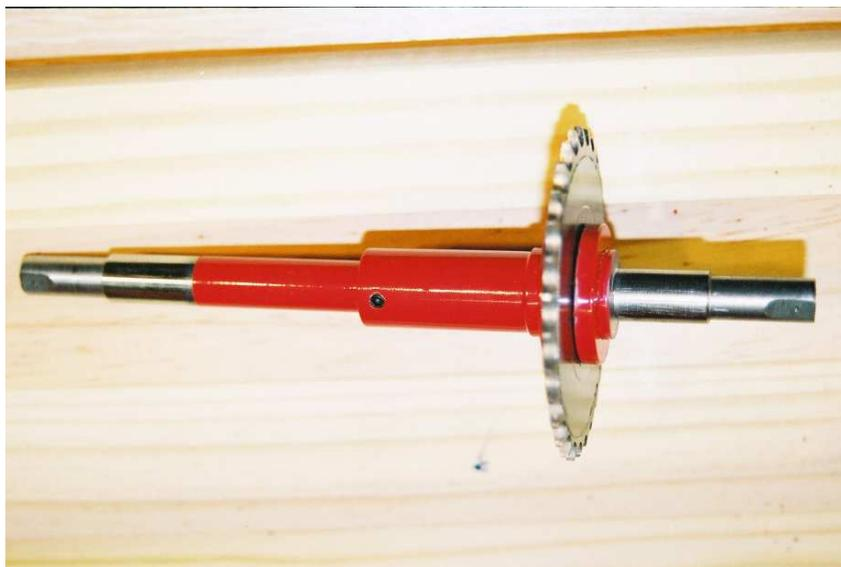
The back axle and differential ready to fit to the rear suspension. The parts for this were shown in the April journal, photo #3.
