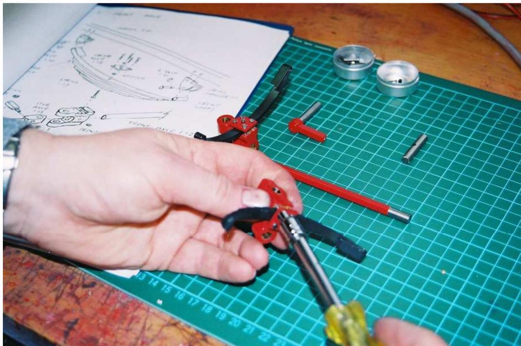
Assembling the front spring to the stub axle.
