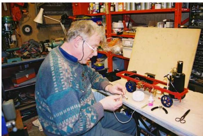
This was fairly easy, as all the pipes are pre bent to shape. Only small adjustments were necessary to get a good fit. Other fittings are also installed at this stage, such as a steam lubricator, supplied, and pipe lagging if you want to add it. This is simply cotton based string wound tightly around the pipe and super glued in place taking care not to glue any gland or joining nuts at the same time.
