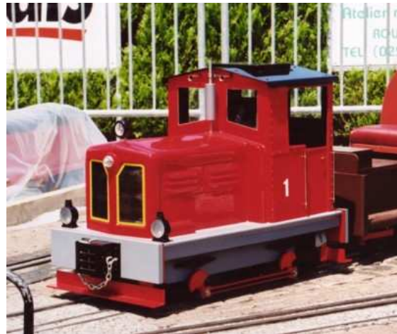
Petrol hydraulic rack engine
